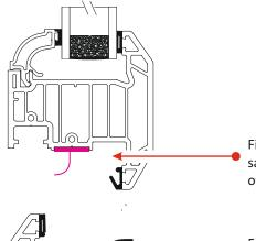
Fit a Sash Spring to the sash on the center line of the stay fixing area
