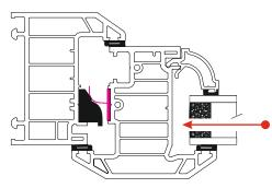
It may be necessary to pack the sash/glass at this point as shown
